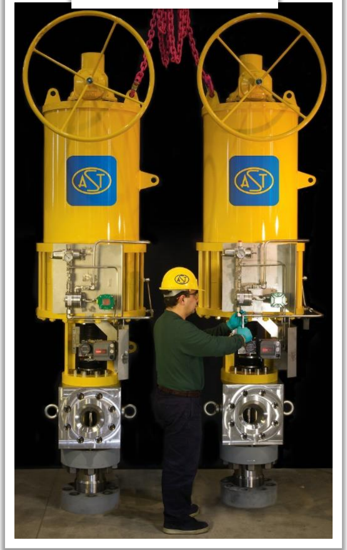
CV-870U – DN 8" PN 320 Carbammate Recirculation Body: AISI 316L Urea Grade Trim: HVD1- Duplex Stainless Steel
